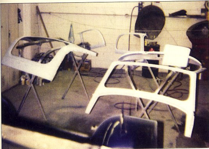
All body panels were stripped, primed and painted off the car, again using Sikkens products. Although the shop has a spray booth, Steve painted some of the parts in his workspace, after wetting down the floor.
