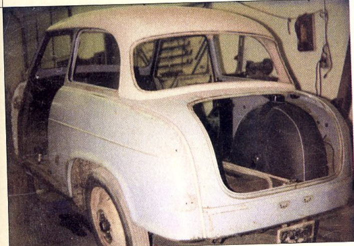
With the car supported on jackstands, disassembly was straightforward. Removing the windows without damaging the gaskets or cracking the glass required the use of dish soap as a lubricant, and gentle pressure.
