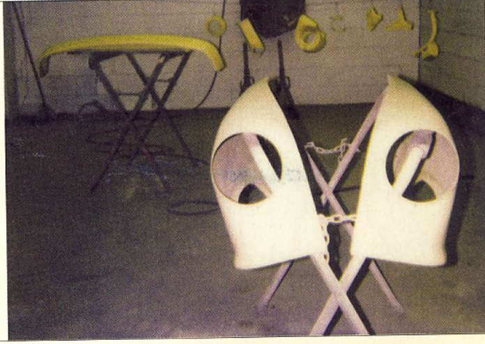
About a teaspoon's worth of filler, to fill in a dent in a front fender, was all that the car needed. A paint supplier matched the original colors, using areas of the car that had been protected from fading.
