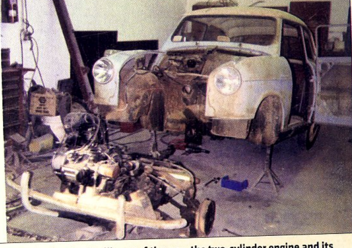
With the hood and grille out of the way, the two-cylinder engine and its attached gearbox could be dropped out. The whole assembly attaches to the tubular backbone of the car with four large bolts.
